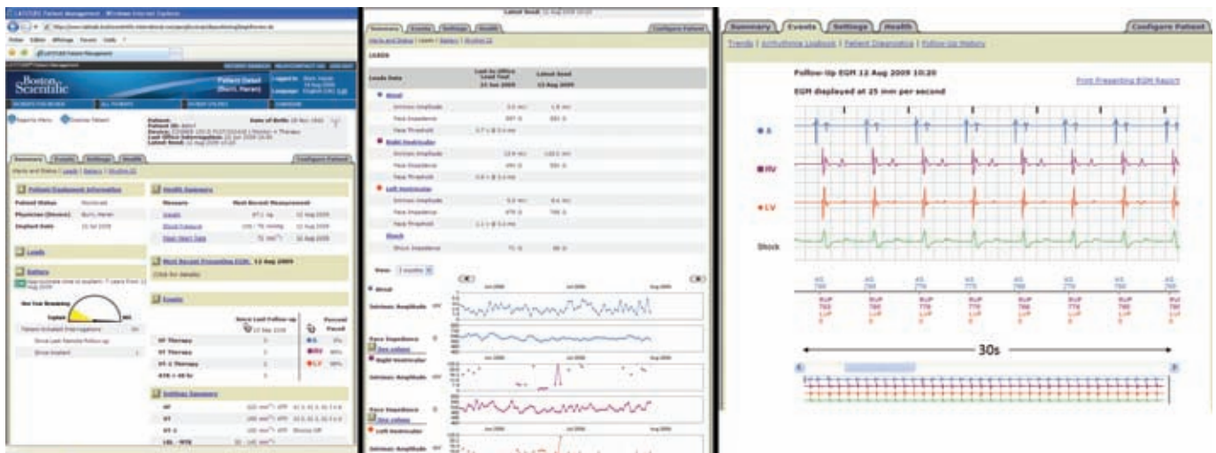
The panel on the left is a print screen of the overview of the device data and settings. The middle panel gives details of lead measurements and their trends. On the right, a realtime 30 seconds electrogram shows the patient's current rhythm. Source: Boston Scientific.
